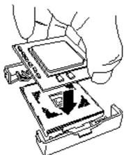
Note: Be aware of CPU direction. Pin layouts on two corners among four differ from others to prevent an incorrect insertion. Confirm the pin mark and pin layout on the socket, and insert the CPU correctly.
